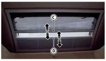
Fig. 6.10 - Tilting skylight with fly screens and window shades
