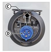
Fig. 6.29 - 220 V power supply socket
