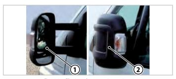
Fig.4.1 - Closing the rear view mirror
