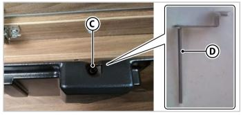
Fig.6.16 - Releasing a Type A electric bed
