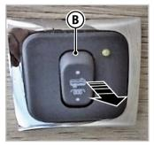
Fig.6.36 - Heater switch
