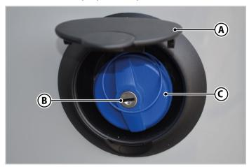
Fig. 6.31 - Refilling the white water tank
