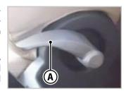
Fig. 3.4 - Backrest adjustment control
