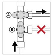
Fig.6.25 - Opening and closing the taps
