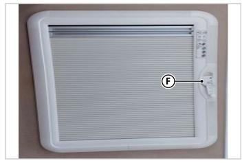
Fig.6.7 - Tilting skylight - Type B
