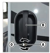
Fig.5.1 - Opening/closing the entrance door from the outside
