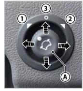
Fig. 3.1 - Adjusting the mirrors
