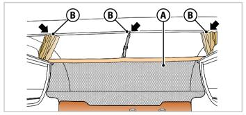
Fig. 6.18 - Protective net for pull-down bed over dinette
