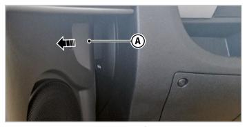
Fig. 5.8 - Bonnet opening lever - Type A
