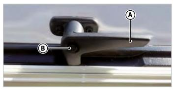
Fig.6.2 - Window locking lever
