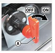
Fig.6.30 - Battery disconnect switch
