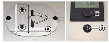
Fig. 6.15 - Command for pull-down bed over dinette compartment
